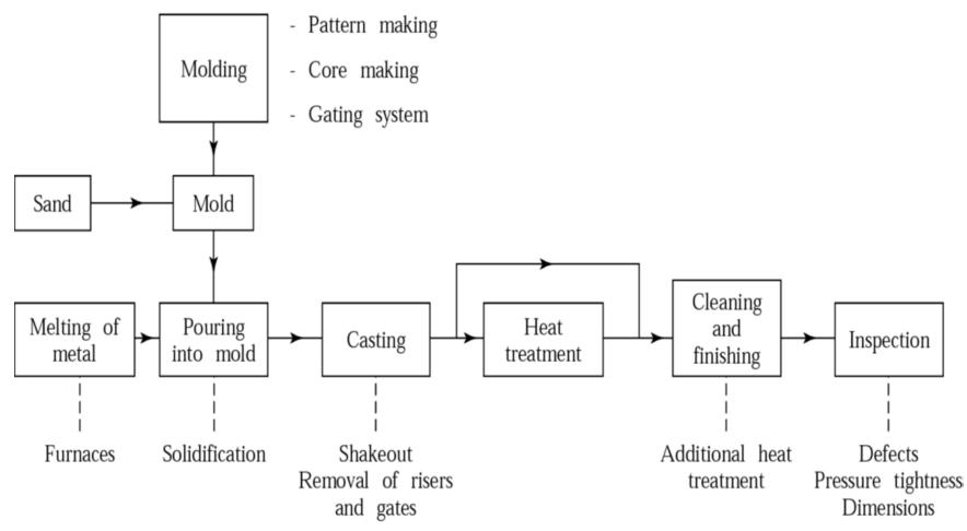
• A line diagram showing sand casting steps
